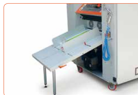
Delivery table with air fans.
